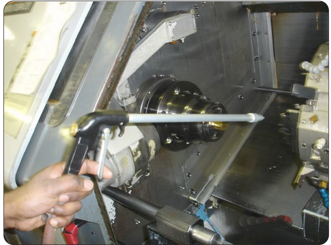
Hand Comfort button Gun is Used for blowing off metal chips during a drilling operation.
